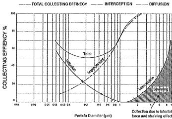
The key is where the Impingement drops off just as the Diffusion increases. It is that range from slightly below to slightly above 0.3 microns that is the least effective. All other sizes are more effective.
